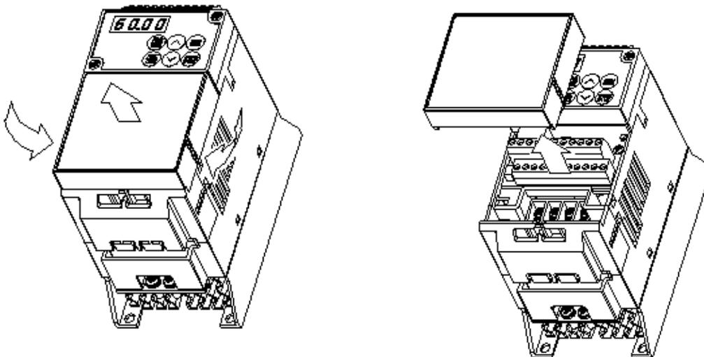
Fig. 1-3-1 Removing the control terminal block cover
