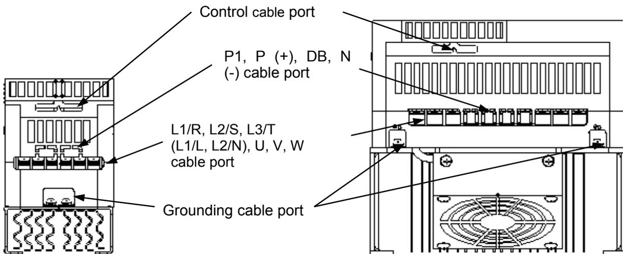
A barrier is provided in the main circuit terminal block cover for the P1, P (+), DB and N (-) cable port. Cut the barrier using nippers or the like before wiring.
