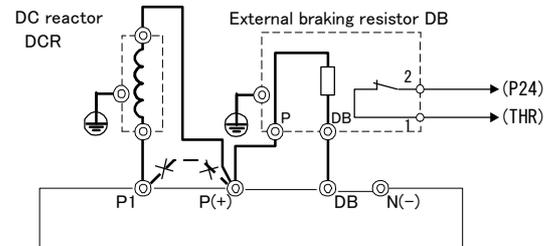
Fig. 2-3-2 Connection diagram
