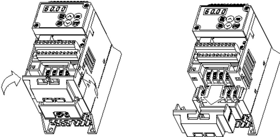
Fig. 1-3-2 Removing the main circuit terminal block cover
