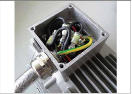
Fig. 11: Wiring on the motor connection box
